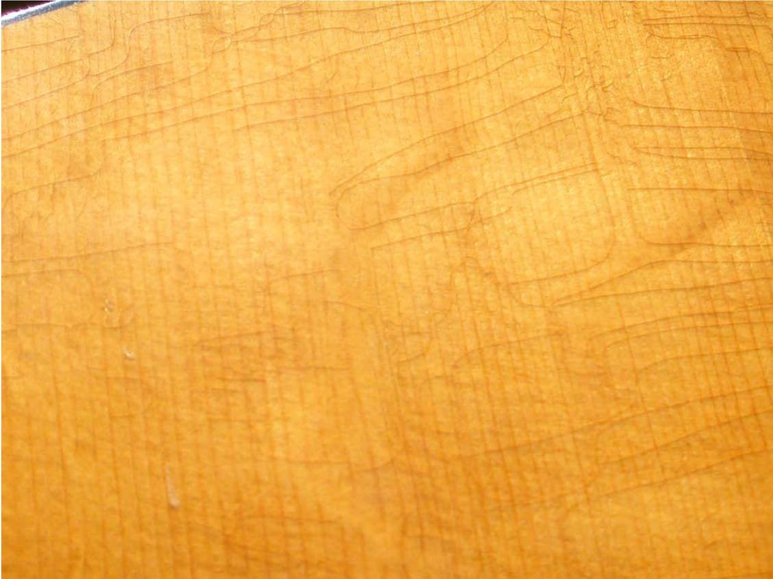
**Figure 51** shows the cracked varnish coating on a classical guitar after being exposed to 5° F.
