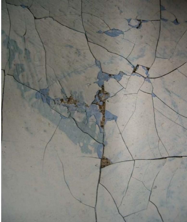
**Figure 66** shows a detail of a painting by Henry Cliffe, painted in 1959. The paint shown in this detail is lead white with zinc in it. Note the severe cracking and inter layer cleavage. This is mechanical damage due to rolling and not to moisture or temperature effects. (Photograph courtesy of Richard Saltoun and taken by Steve Gayler)
